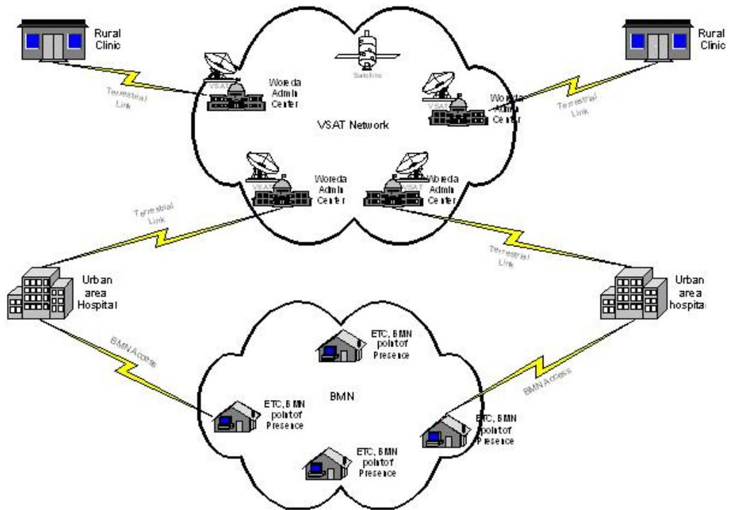
Figure 2: Logical WAN design based on BMN and VSAT networks alternative one.
