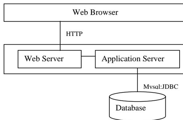
**Figure 5: Architecture of BTS**
