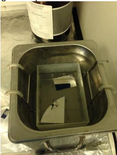
Figure 5. Development using ultrasonic agitator.
