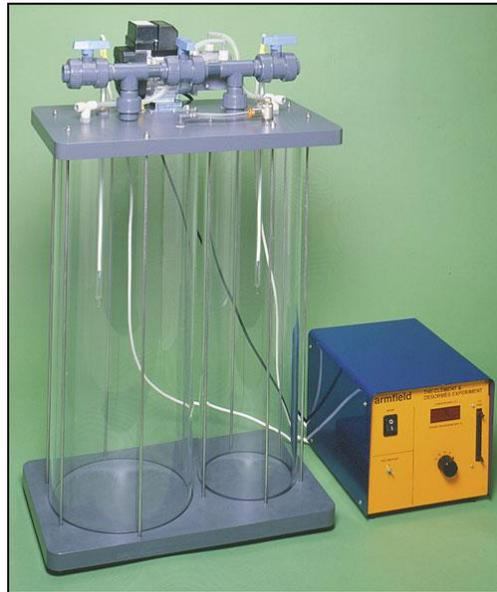
**Figure 1:** TH5 Expansion Processes of a Perfect Gas Apparatus, Armfield Limited.
