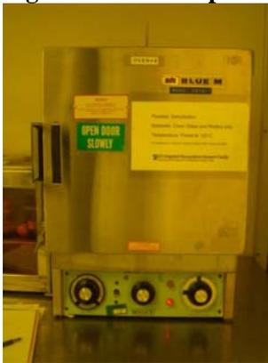
**Figure 4.10 Oven used for soft-bake process (made by BLUE M).**
