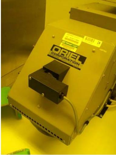
**Figure 4.11 UV light machine made by Oriel.**
