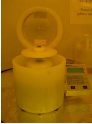
**Figure 4.8 Spinner used for spin-coating (made by Laurell technologies).**
