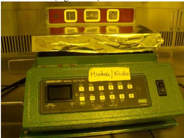
**Figure 4.19 Leveled hot plate (95 °C) used for PEB (Courtesy of Madou's Lab at UCI).**
