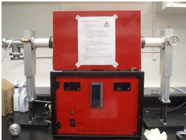
**Figure 4.23 High temperature vacuum/inert gas atmosphere furnace made by RD Webb Company.**
