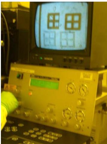
**Figure 4.18 Alignment marks matching process (mask alignment process II).**
