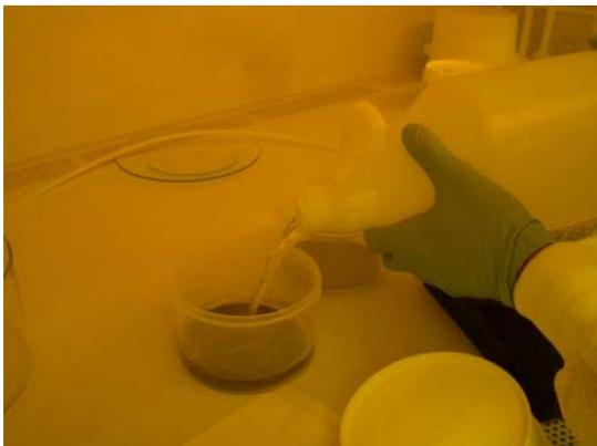
**Figure 4.13 Developing process using SU-8 developer.**
