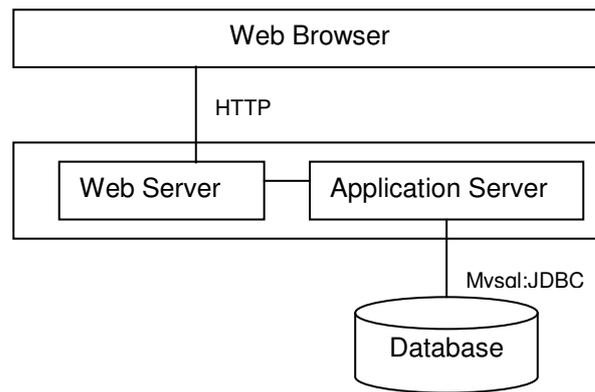
Figure 5: Architecture of BTS
