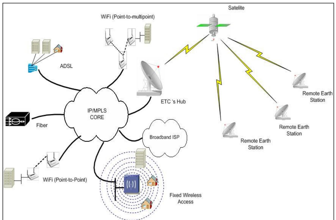
Figure 4: ETC’s Broadband Integrated Infrastructure for e-Health Applications
