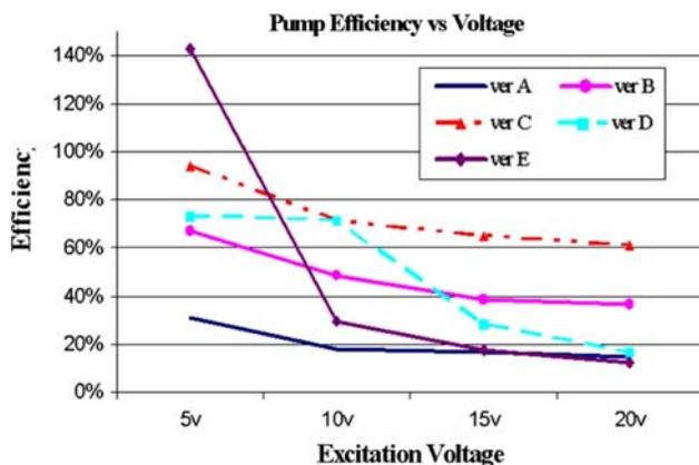
**Fig. 10** Comparison of micropump efficiency between theoretically predicted and experimental flow rates in the various MHD pump configurations. **a** 5 V, **b** 10 V, **c** 15 V, **d** 20 V. The efficiency of a given design is given as  $(1.0 - (\text{theoretical value} - \text{experimental value})/\text{theoretical value}) \times 100.0$
