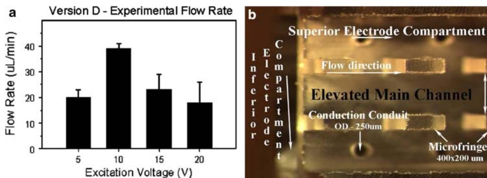
**Fig. 7** **a** Flow rate of the BIRS MHD micropump (version E) under DC excitation; **b** micrograph of BIRS MHD micropump. Main channel and electrode compartments are shown
