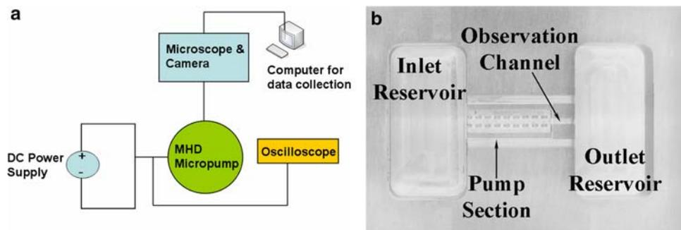
**Fig. 2** Experimental set-up. **a** Schematics of the experimental set-up consisting of power supply, micropump, microscope and camera as well as data acquisition. **b** Location of inlet and outlet reservoirs, pump section and the observation channel. Here, the pump sections are sealed from the external through glass cover-slips. Custom teflon insulated platinum electrodes 200 μm in diameter are powered using
