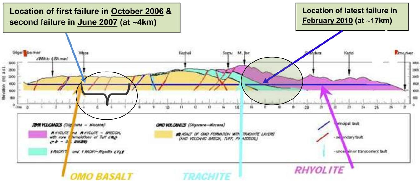
**Figure 4.** Cross-section of the tunnel showing multitudes of fault lines [6,7]. Later failures showed that there were still more fault lines unforeseen at the beginning of the project. Image taken S.E.L.I.’s public report from [6,7].
